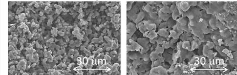
(a) Before absorption (b) After absorption at 550°C
