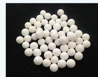
Photo:  $\phi=5\text{mm}$  spherical LS pellet from Toshiba Corporation
