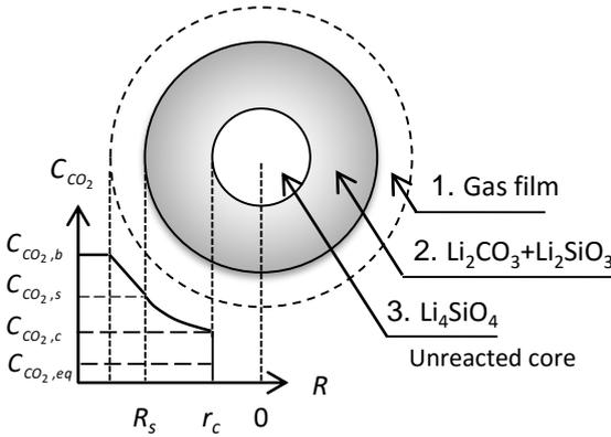
1. Rate of CO<sub>2</sub> mass transfer through the gas film
